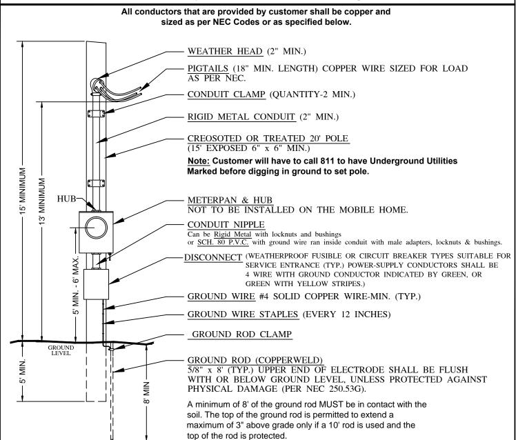
This drawing depicts a typical installation. If the customer's proposed service installation will be located within 3' of a window, door, porch, balcony, ladder, stairs, fire escape or similar location, CONTACT SLECA.
